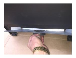
2. Locate the bottom of the adapter with the 2 bends under the bottom rear of the stove which will locate and secure the bottom part of the adapter, align the 2 key holes on the adapter with the 2 screws on the back of stove which was loosened above and fasten 2 screws up tight.
