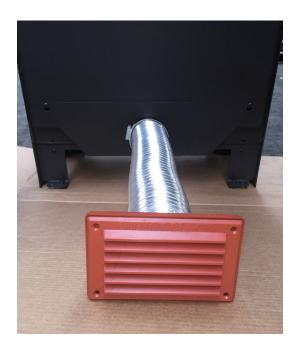
3. From the hearth level to the centre of the outside air intake spigot on the stove is; Avance 500 tall is 140mm Avance 500 short 70mm Avance 400 is 110mm With the 3" / 76mm hole pre-cut through the outside wall you can now push the flexi tube through the hole from the outside and fasten the grill onto the outside wall with 4 screws
